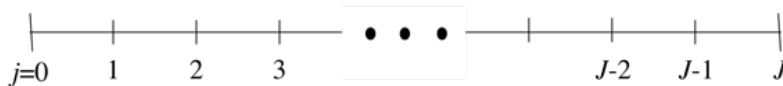
Figure 15.4: An outflow boundary condition must be specified at j = J in this finite and non-periodic domain.
