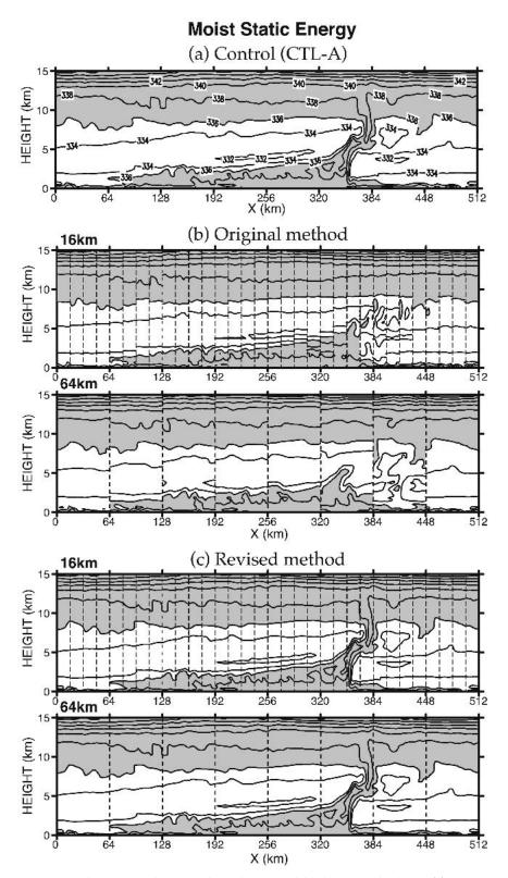
FIG. 4. Vertical cross sections of moist static energy divided by  $c_p$  obtained from (a) Control (CTL-A) and the MMF experiments with the (b) original and (c) revised methods using (upper) 16- and (lower) 64-km horizontal grid sizes of the LSDM. The areas with higher values than 336 K are shaded. Contour interval is 2 K. The dashed lines in (b) and (c) represent the LSDM grids.
