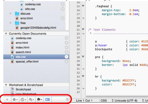
The buttons and popup menus at the bottom of the sidebar are commands that give you quick access to project functions. You can use these commands to add new items, create new files and folders, open existing files and folders, reveal them in the Finder or navigate to them in the Terminal, limit the kinds of files which appear in the project list, and navigate through your disks and folders.
