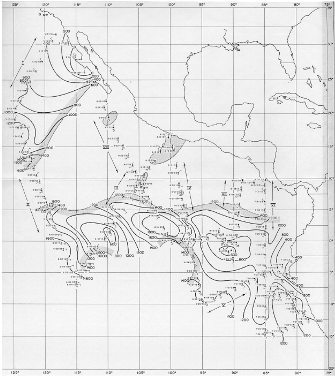
Figure 1.1: Plot of inversion base height from 1952 cruises of the Horizon. Figure taken from Neiburger (1961)
