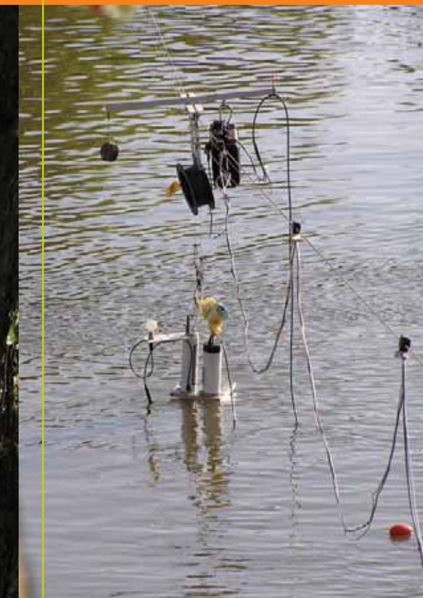
Water quality and flow sensors positioned at the surface of the river.
