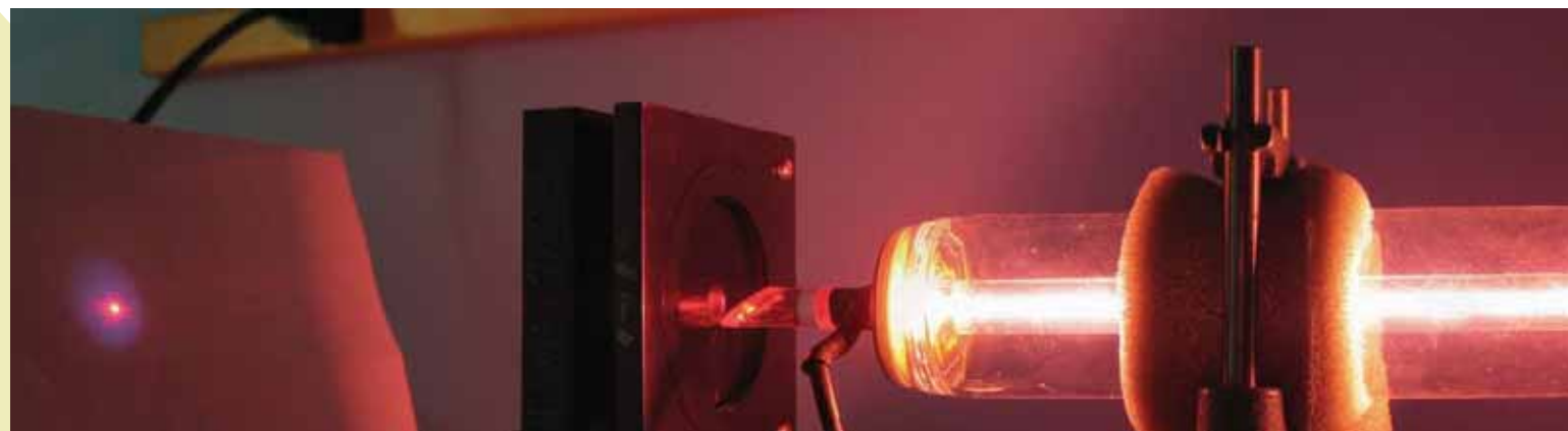
Helium Neon laser. Photo: Marco Molinaro
