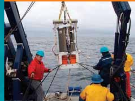
On March 16, 2006, the second-generation version of an underwater, robotic DNA lab called the Environmental Sample Processor (ESP) was deployed in Monterey Bay, Calif. Photo: (c) 2006 MBARI
