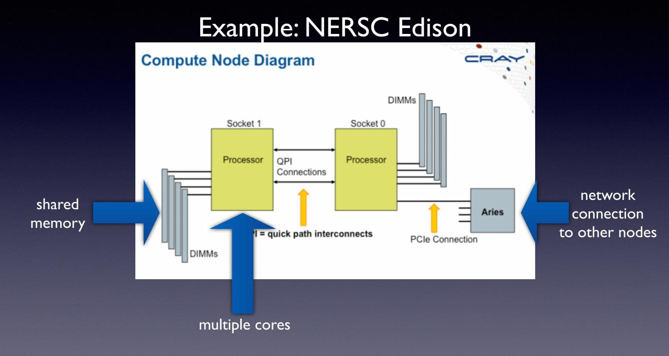
2 processors x 12 cores/processor = 24 cores/node
