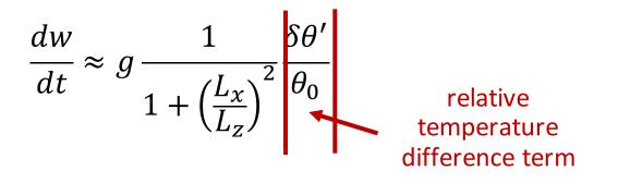
$\delta\theta'$  is different than  $\theta'$  in that it is the temperature difference between the center of an updraft and its immediate surroundings, rather than an arbitrary base state
