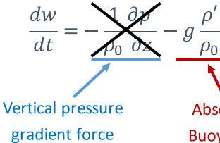
Absolute Buoyancy Neglecting the vertical pressure gradient force: how valid is this assumption?
