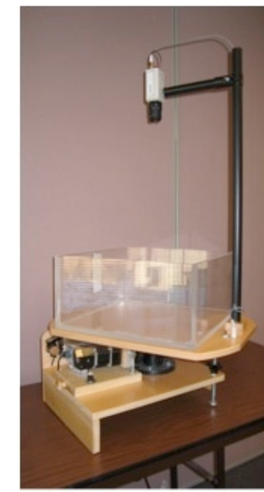
Figure 2. Rotating tank with bottom dimensions of 16x16 inches.
