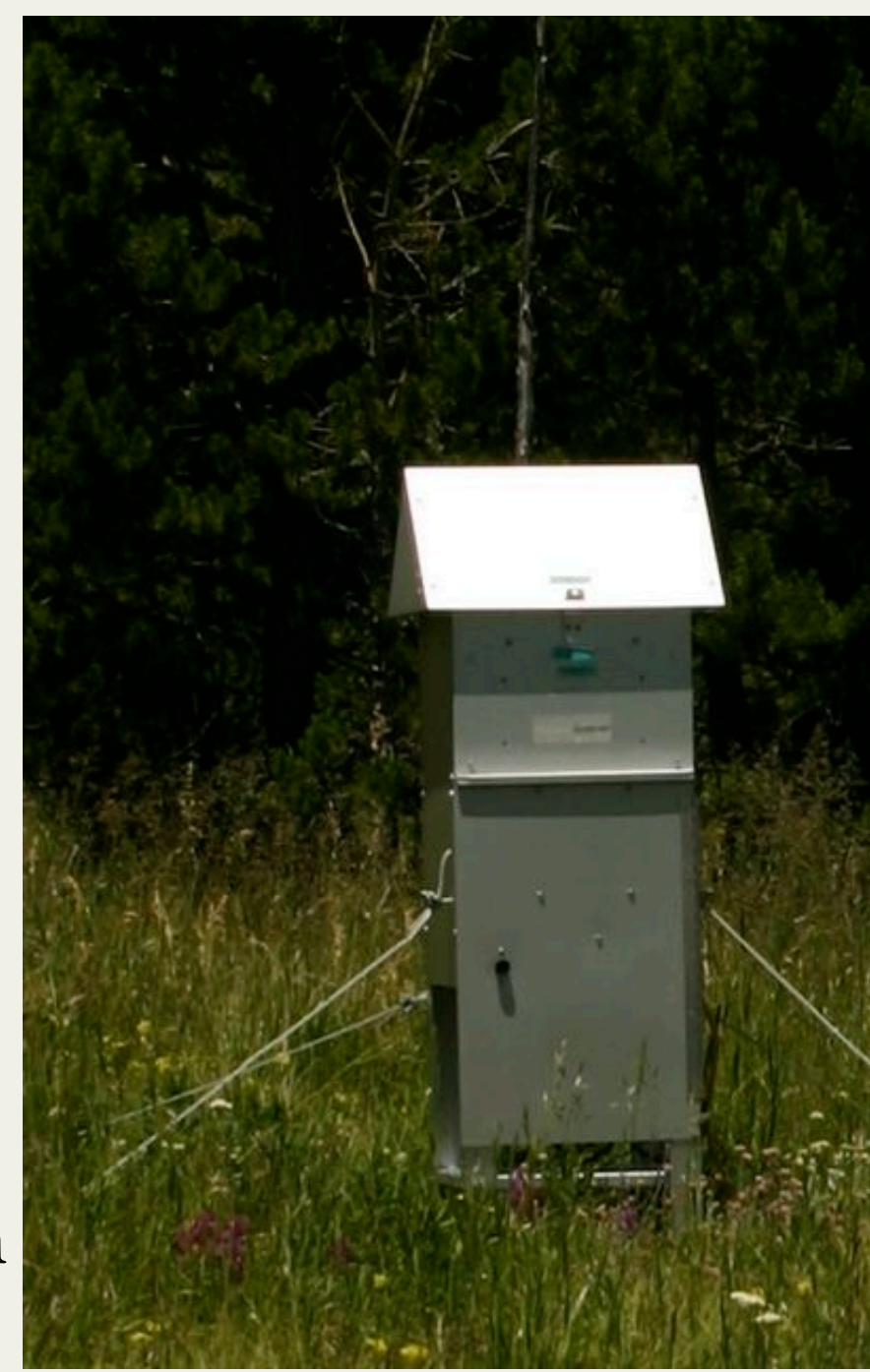
Figure 1: An example of a filtering device used to take 24 hour samples in the field.
