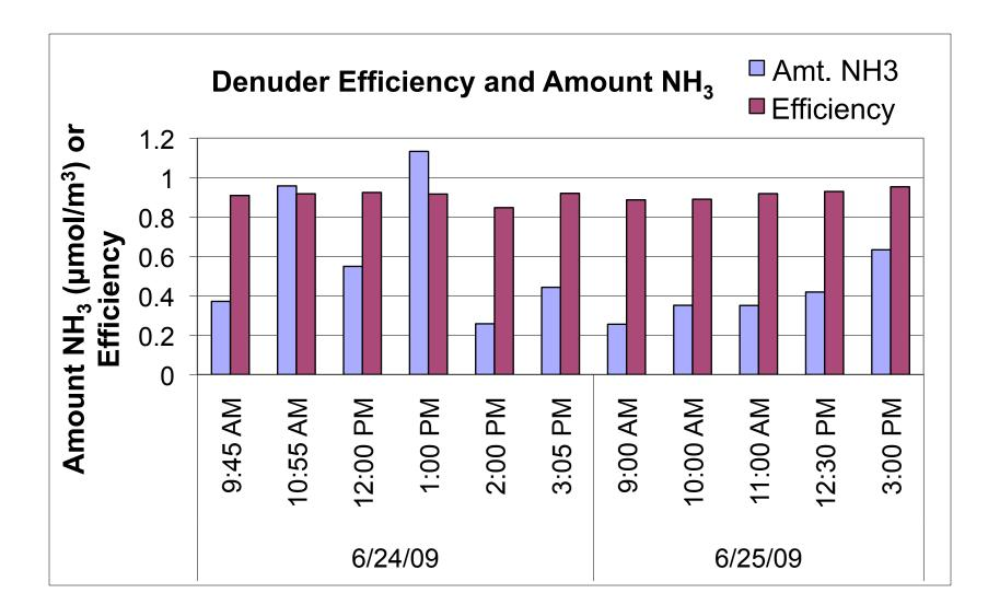
•The concentration of ammonia varied by location and method for sampling. The dynacalibrator (an instrument that generates ammonia in the lab) provided the highest concentration of ammonia, resulting in higher efficiencies than in the lab or field
