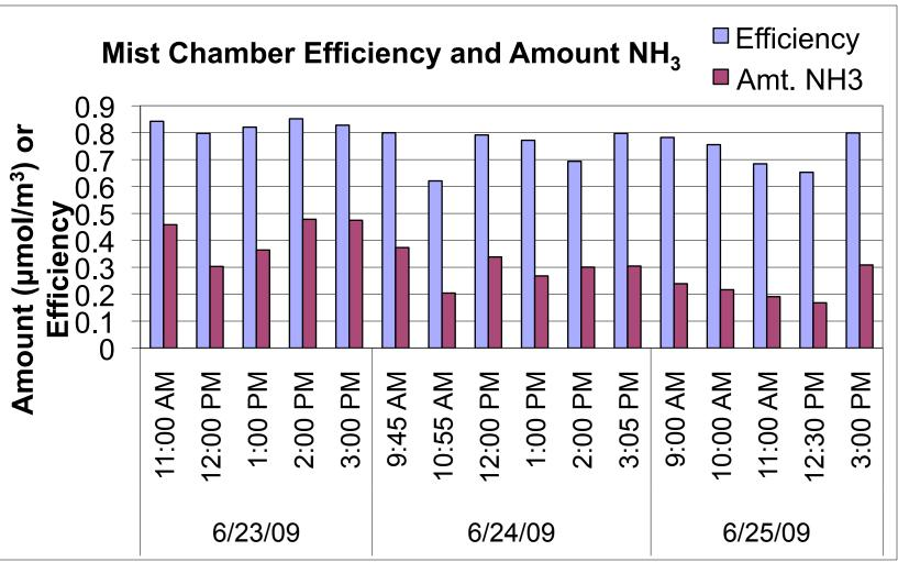
•Denuders that were setup near the lab also measured the amount of ammonia, which was compared to the ammonia measured by the mist chamber. Most of the time the denuder collected a higher concentration of ammonia
