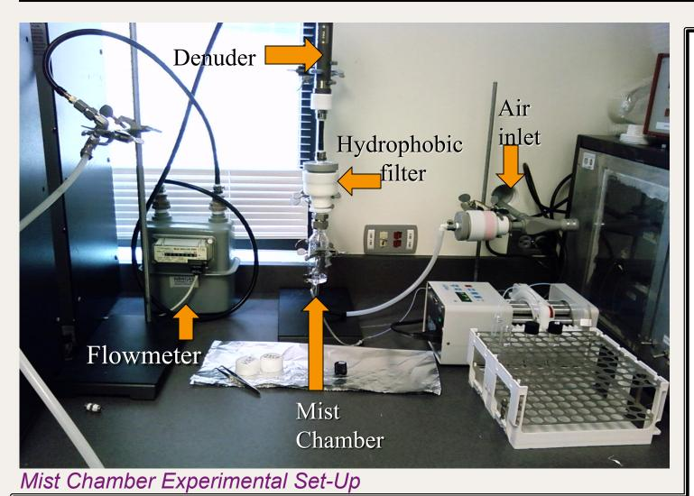
•After initial experimentation, it was determined that 10 mL of trapping solution would be used for the mist chamber •For ammonia, the trapping solution used had a pH of about 2.00 and was made of HCl, DI water, and LiBr (to be used as an internal standard)
