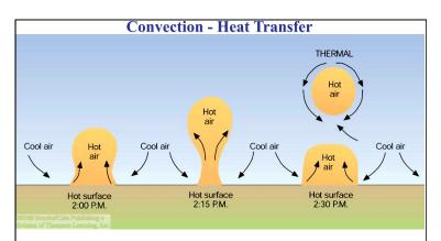
Convection is heat energy moving as a fluid from hotter to cooler areas.
