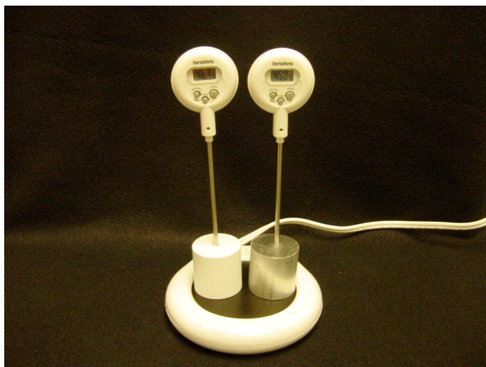
Two cylinders on the hot plate. After they are warmed, they will be set aside to cool. Which will cool fastest—the white or the silver?
