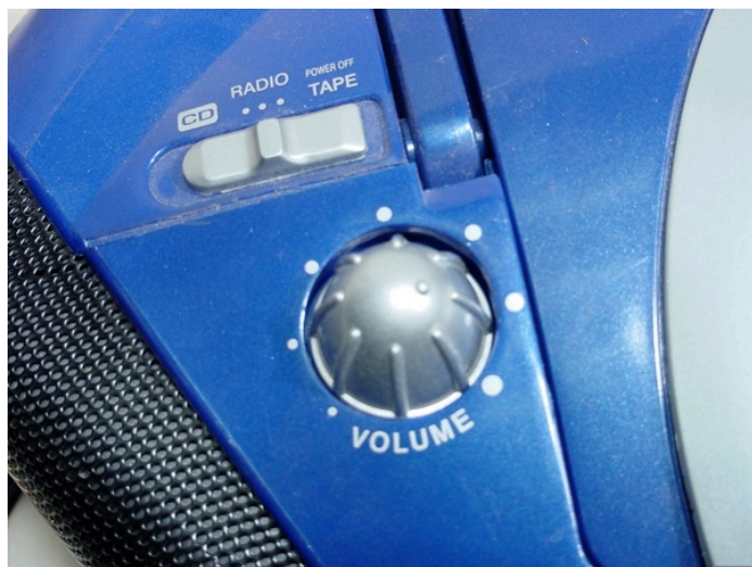
This CD/radio/tape player uses energy even when it is turned off. The energy it uses depends on the function chosen.
