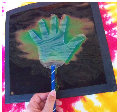
The plastic absorbs and reradiates thermal energy, keeping the sheet below warmer.
