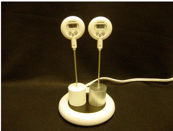
Two cylinders on the hot plate. After they are warmed, they will be set aside to cool. Which will cool fastest—the white or the silver?
