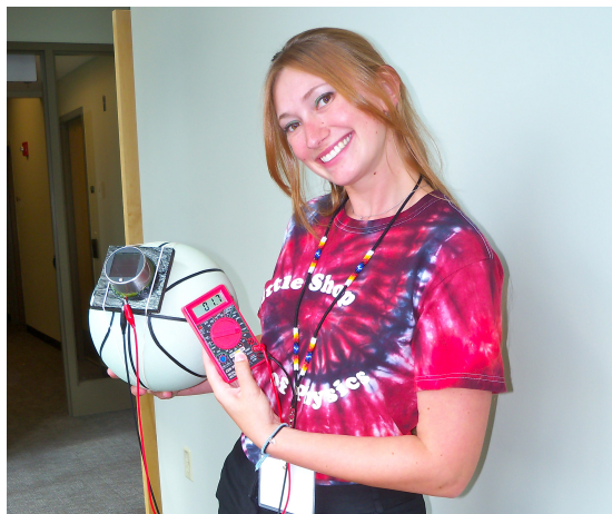
As the basketball is tipped in relation to the sun, the solar cell will generate more or less current which can be measured by the multimeter.
