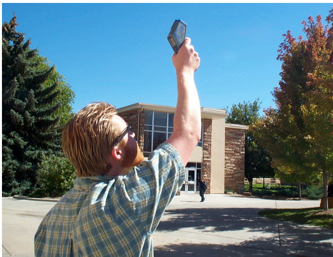
Taking the temperature of the sky. On this clear Colorado afternoon, it was a frosty -30^{\circ}\text{C} .
