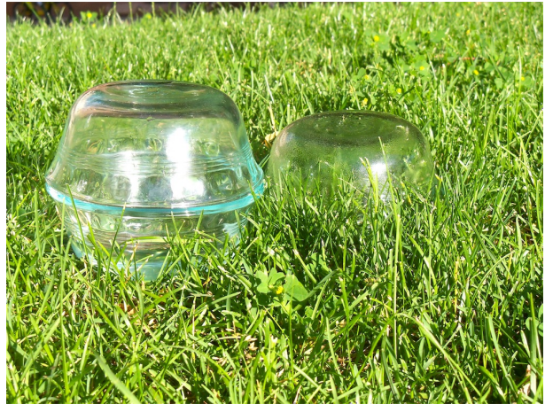
There is more condensation on the glass over the grass (right) than over the cup of pure water (left)
