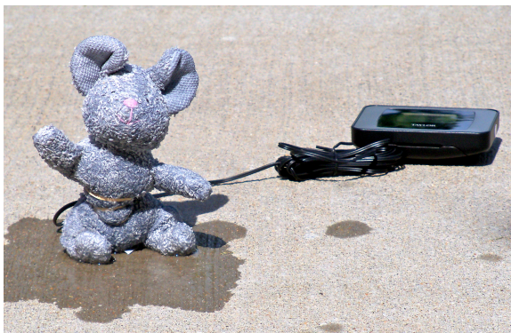
The indoor/outdoor thermometer takes two readings: one of the "wet" temperature and one of the "dry."
